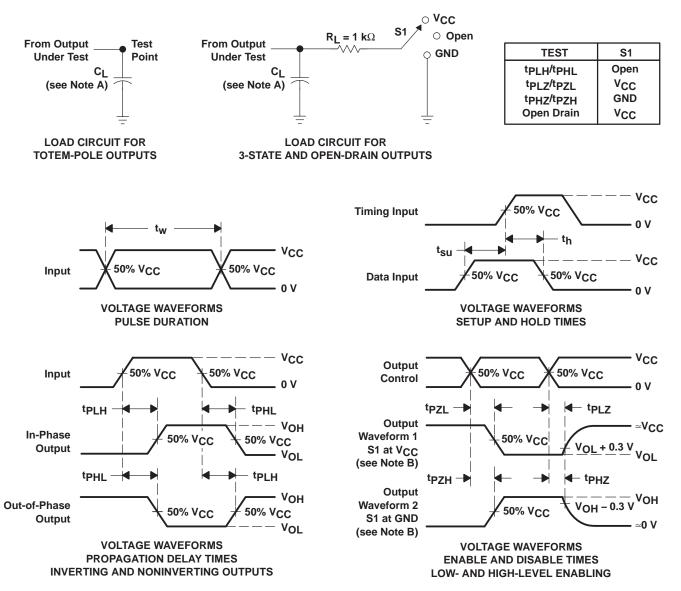
NOTES: A. C<sub>L</sub> includes probe and jig capacitance.
