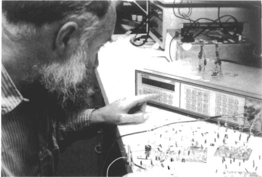
Figure 3.2. Bob uses carefully selected precision resistors to model the resistance of the metal runs of a FET op amp. (Photo by Steve Allen.)
