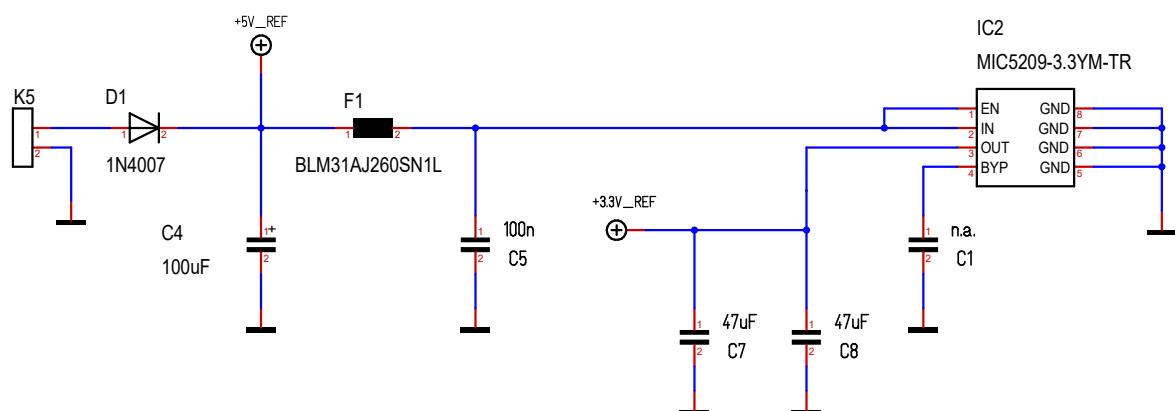
The output capacitor should have an ESR (equivalent series resistance) of about 1Ω and a resonant frequency above 1MHz. Ultra-low-ESR capacitors can cause a low amplitude oscillation on the output and/or underdamped transient response. Most tantalum or aluminum electrolytic capacitors are adequate; film types will work, but are more expensive. Since many aluminum electrolytics have electrolytes that freeze at about -30°C, solid tantalums are recommended for operation below -25°C.
